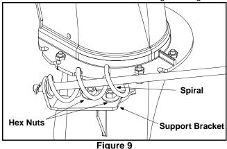
Adjust the support bracket inward or outward so that the spiral is fully engaged in the notches on the chute before retightening the hex nuts.
